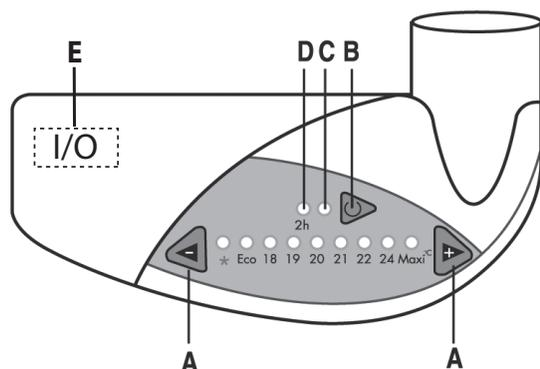
After connecting your appliance to the electrical installation, put the switch located at the back of the control on the [I] position to turn it on.
